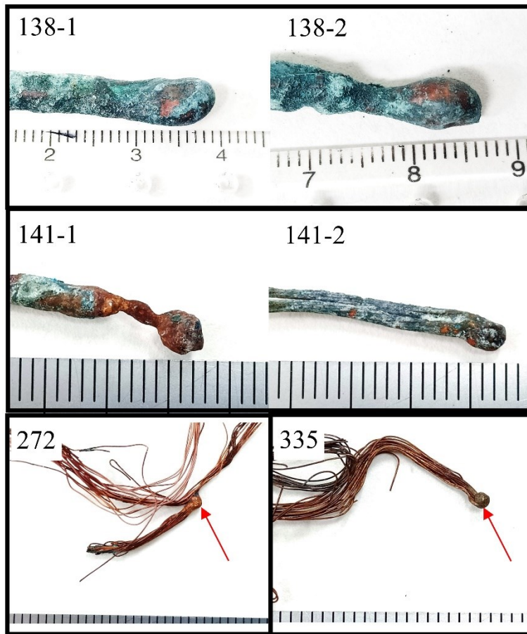
Fig. 4.4 The melted marks on copper wire collected from the real fire sites
