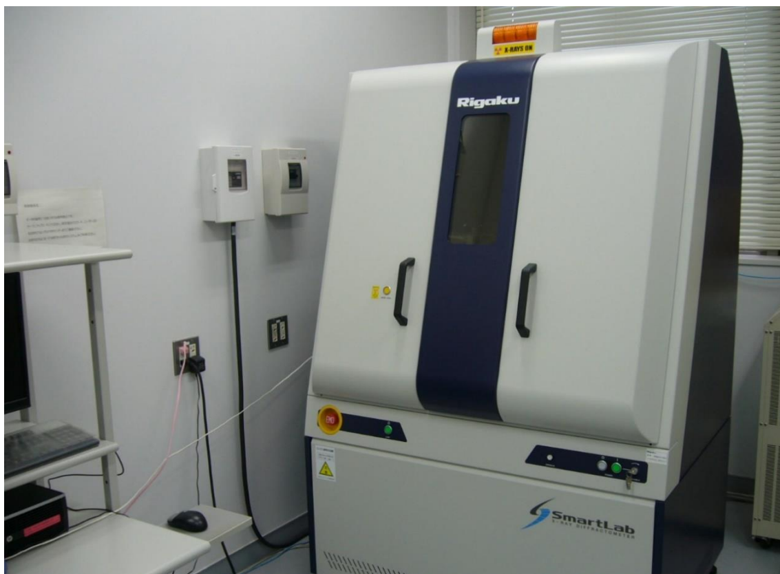
Figure 3-2. XRD measurement facility (SmartLab, Rigaku Co.) at the Center for Advanced Instrumental Analysis in Kyushu University
