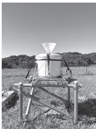
図 1 a) バルク降水採取器, b) 降雪採取器 (11月～4月; 北海道演習林) Figure 1 a) bulk precipitation collector, b) collector for snowfall (from November to April in Ashoro Research Forest).
