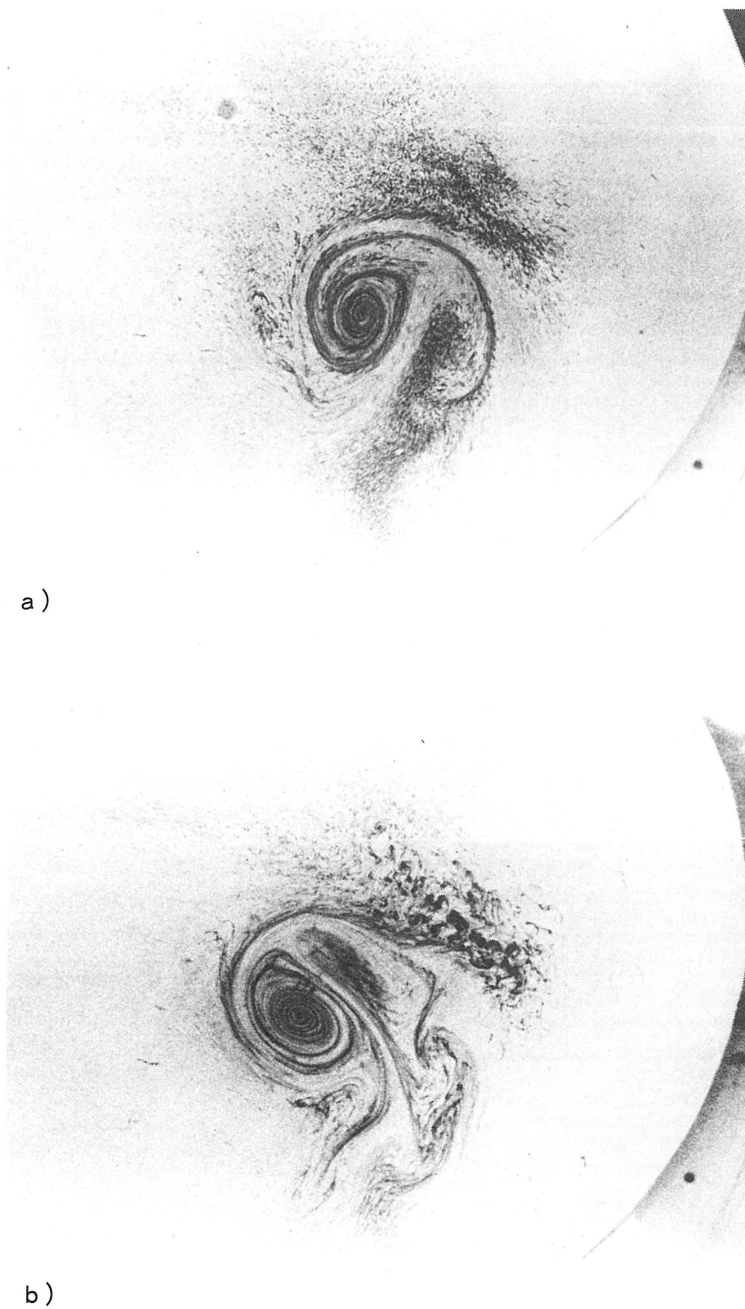
Fig.9 Flow patterns generated by a fixed ice cube, a) t = 11 T , b) t = 19 T : H_0 = 8\text{cm} , \gamma = 1/4 , T = 17\text{ sec.}
