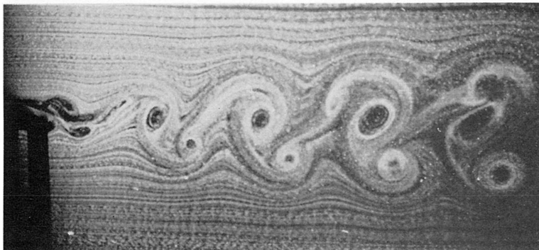
Fig. 9 Vortex street in the case of downstream cylinder oscillating at R_c=3 \times 10^3 , a/d=0.3 and s/d=1.5 . S_c=0.32 , S_c/S_v=2.0
