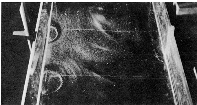
Fig.4. Plan view of induced streaming and a particle wave formed on the bottom floor of a water tank 50 cm wide. \nu = 0.41 \text{ cm}^2/\text{s} .
