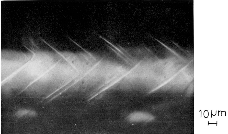
Fig. 19(c) Impure MRC(0.2) ( \chi=25^\circ , \lambda=37^\circ ) deformed by slip with many twin bursts.
