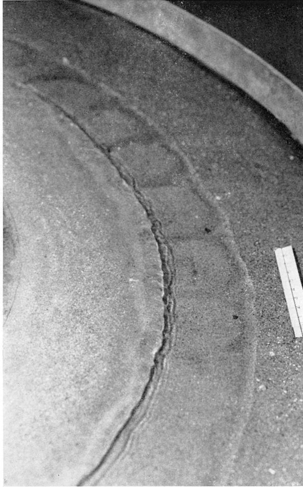
Fig. 4. Bird's-eye view of sand petals. d=4.0 cm, f=2.57 Hz, \theta=9^\circ , t=17 min., scale length=10 cm.
