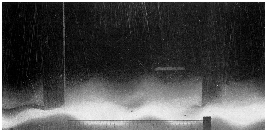
Fig. 7 Sand-bed scour around a square cylinder at left with the side 3.00 cm long. Distance from a circular cylinder at right is 23.0cm: Scale unit in cm. a=6.59 cm, f=0.714 Hz.
