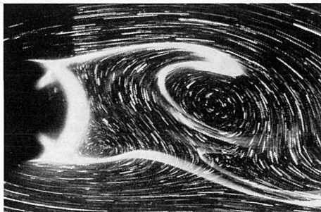
Fig. 5 Streamline and integrated-streakline patterns behind a circular cylinder at R=100 .
