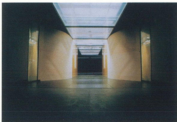
Photo.2 Appearance of the second-contraction system settled in the test section.
