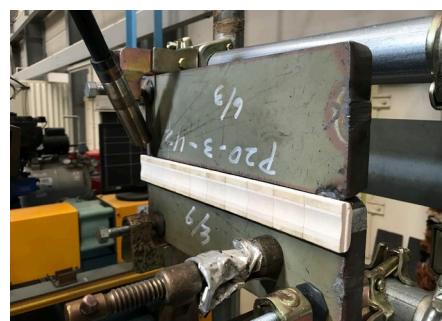
Fig. 7 LAHW-HB with supporting sheet.
