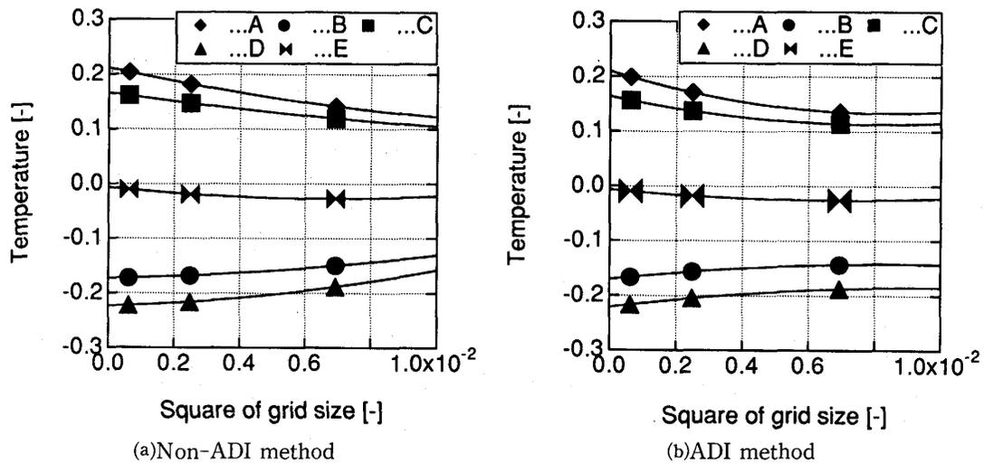
Fig. 6 Extrapolation of temperature at infinitesimal grid size
