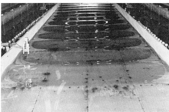
Photo 2.4 Regular wave generated in a canal
