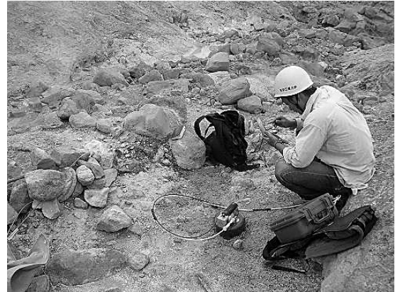
Fig. 4. A photo showing the proceeding of \text{CO}_2 flux measurements from the soil around Aso Nakadake.
