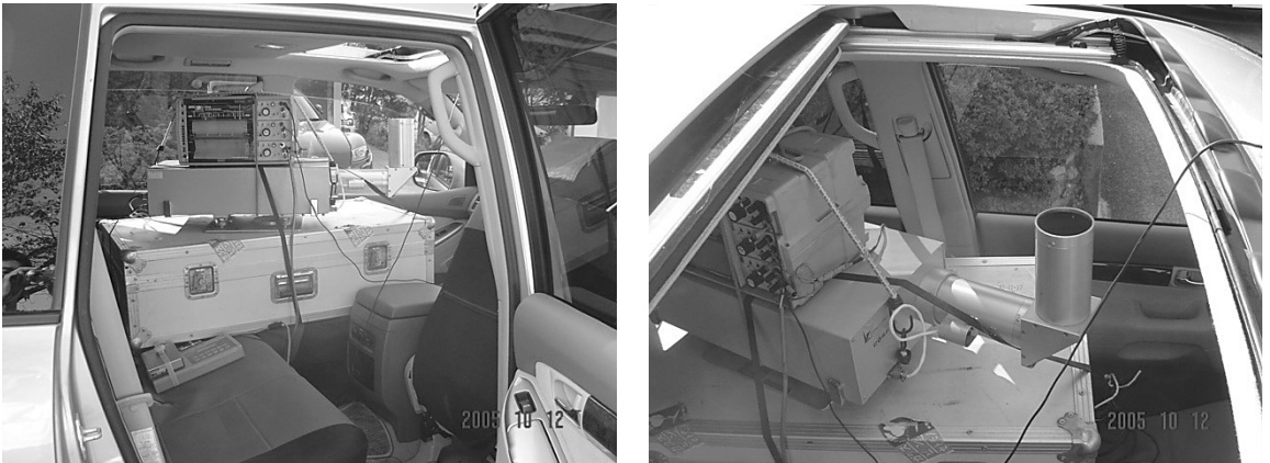
Fig. 7. Photos showing the COSPEC and the data collector installed in a vehicle. A rectangular prism is used to observe \text{SO}_2 column density through the roof window.
