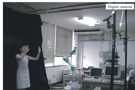
Fig.4 Measurement of human gesture for telecommunication system
