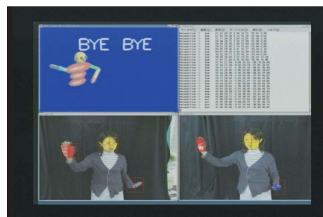
Fig.5 Gesture recognition based on continuous DP matching
