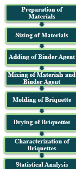
Fig. 1. Process flow for the production of briquettes
