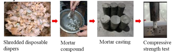
Fig. 3. Experimental Study of Mortar compounds and Comprehensive Strength Test
