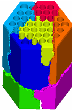
Fig. 4 Part decomposition of a HTTR model
