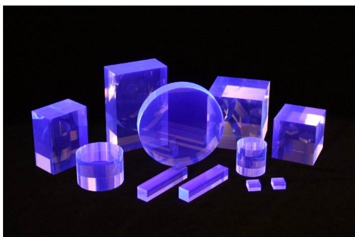
Figure 2.1 Plastic scintillators processed into various shapes. They emit violet to blue fluorescence when irradiated with ultraviolet light [43].
