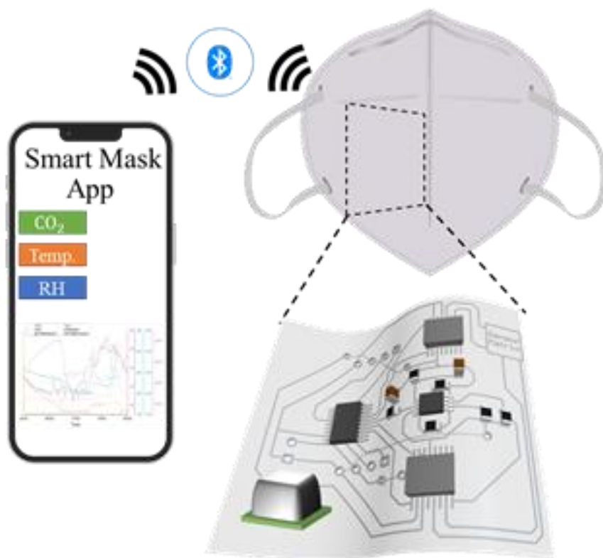
Fig.5.2 The schematic of the smart mask.
