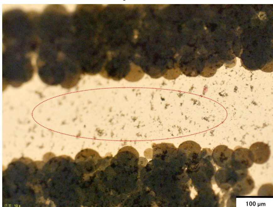
Fig.3.7 Micrographs of the PEG-CB layers (100 μm scale) produced with a micropipette.
