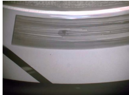
d) Time : 300sec, Cavitation pressure:34kPa(abs.)
