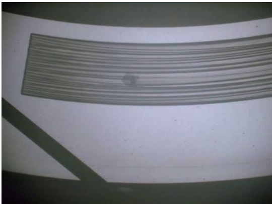
c) Time : 150sec, Cavitation pressure:26kPa(abs.)
