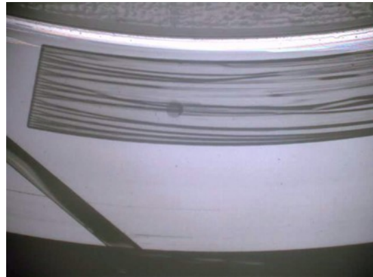
d) Time : 300sec, Cavitation pressure:58kPa(abs.)
