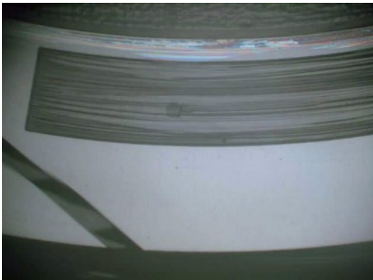
c) Time : 150sec, Cavitation pressure : 72kPa(abs.)
