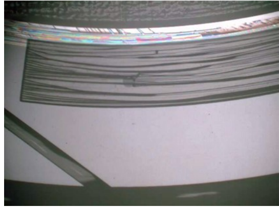
b) Time : 60sec, Cavitation pressure:86kPa(abs.)
