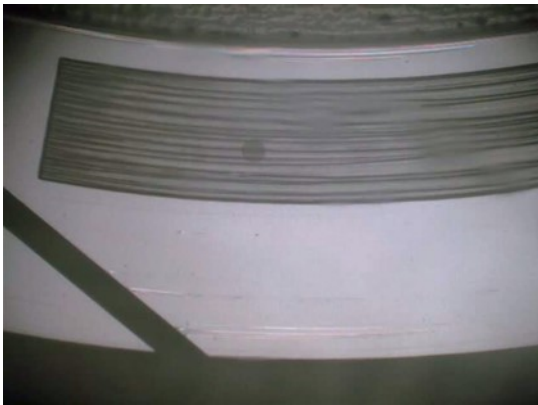
c) Time : 150sec, Cavitation pressure : 69kPa(abs.)
