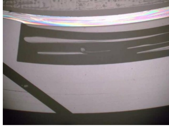
b) Time : 60sec, Cavitation pressure:88kPa(abs.)
