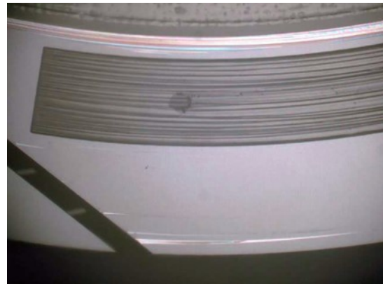
b) Time : 60sec, Cavitation pressure:29kPa(abs.)
