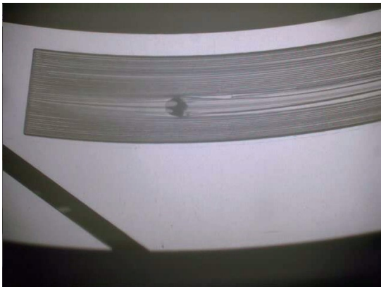
c) Time : 150sec, Cavitation pressure : 18kPa(abs.)
