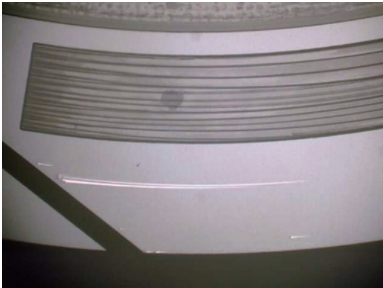
c) Time : 150sec, Cavitation pressure:61kPa(abs.)
