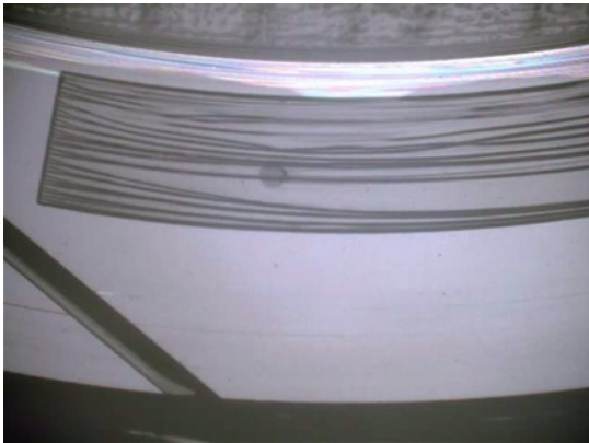
c) Time : 150sec, Cavitation pressure:55kPa(abs.)
