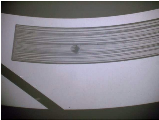
c) Time : 150sec, Cavitation pressure : 31kPa(abs.)
