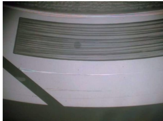
d) Time : 300sec, Cavitation pressure : 69kPa(abs.)
