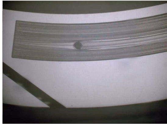
b) Time : 60sec, Cavitation pressure : 21kPa(abs.)
