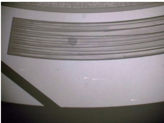
e) Time : 600sec, Cavitation pressure:61kPa(abs.)
