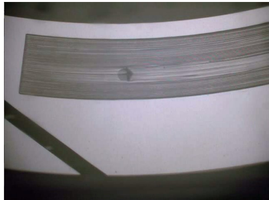
d) Time : 300sec, Cavitation pressure : 17kPa(abs.)
