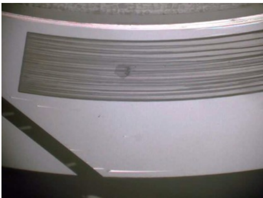
e) Time : 600sec, Cavitation pressure:28kPa(abs.)
