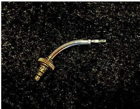
Figure. 2 The image of the fiber tip for Er: YAG laser
