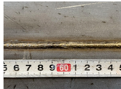
Fig. 1 Example of weld bead appearance (front side, around 600 mm weld length).
