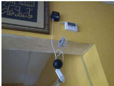
Fig. 4 Location of the thermos-hygrometers: (a) air-conditioner outlet, (b) centre of the room.
