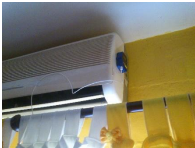
Fig. 4 Location of the thermos-hygrometers: (a) air-conditioner outlet, (b) centre of the room.
