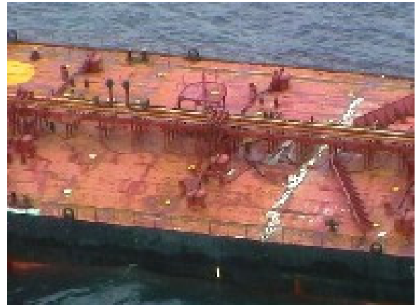
Fig.1 Cracked deck in the tanker Castor (IMO, 2006)
