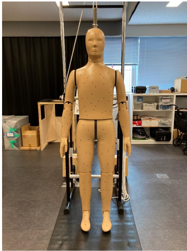
Fig.4-2 Naked thermal manikin
