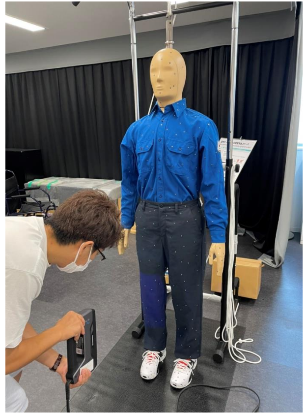
Fig.4-3 clothes thermal manikin
