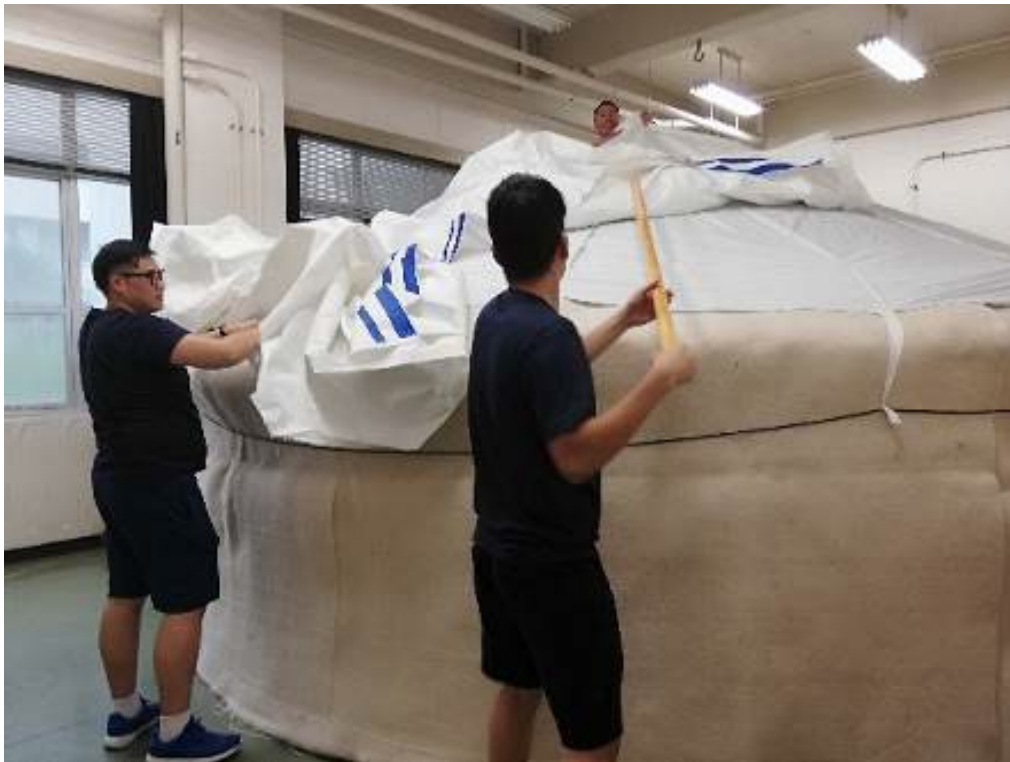
Fig. 3.4 Covering process using a felt sheet
