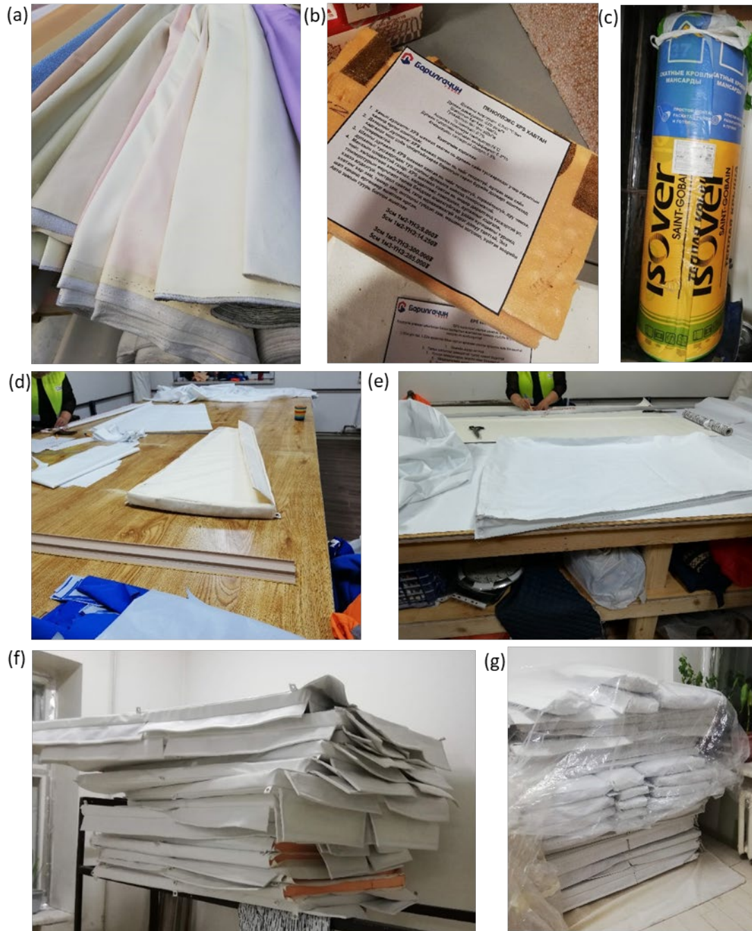
Fig. 3.12 Local materials and manufacturing process: (a) Wall cover fabric; (b) Extruded polystyrene foam insulation board for wall panels; (c) Mineral wool for roof panel; (d) (e) Local manufacturing process; (f), (g) Final locally manufactured panels
