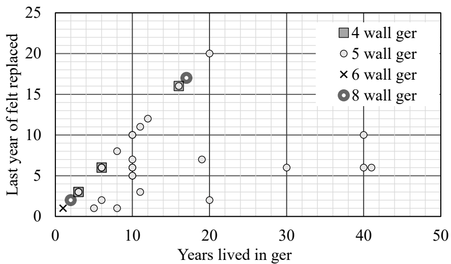
Fig. 2.17 Relationship between the replacement life of felt sheeting and number of years that the respondents have been living in the current ger
