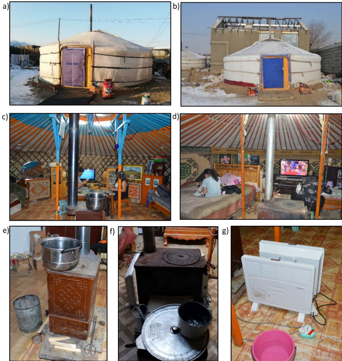
Fig. 4.2 (a) Exterior of Ger A , (b) exterior of Ger B , (c) interior of Ger A , (d) interior of Ger B , (e) ulzii stove used in Ger A , (f) khas stove used in Ger B , and (g) electric heaters used in Gers A and B during Terms II and III
