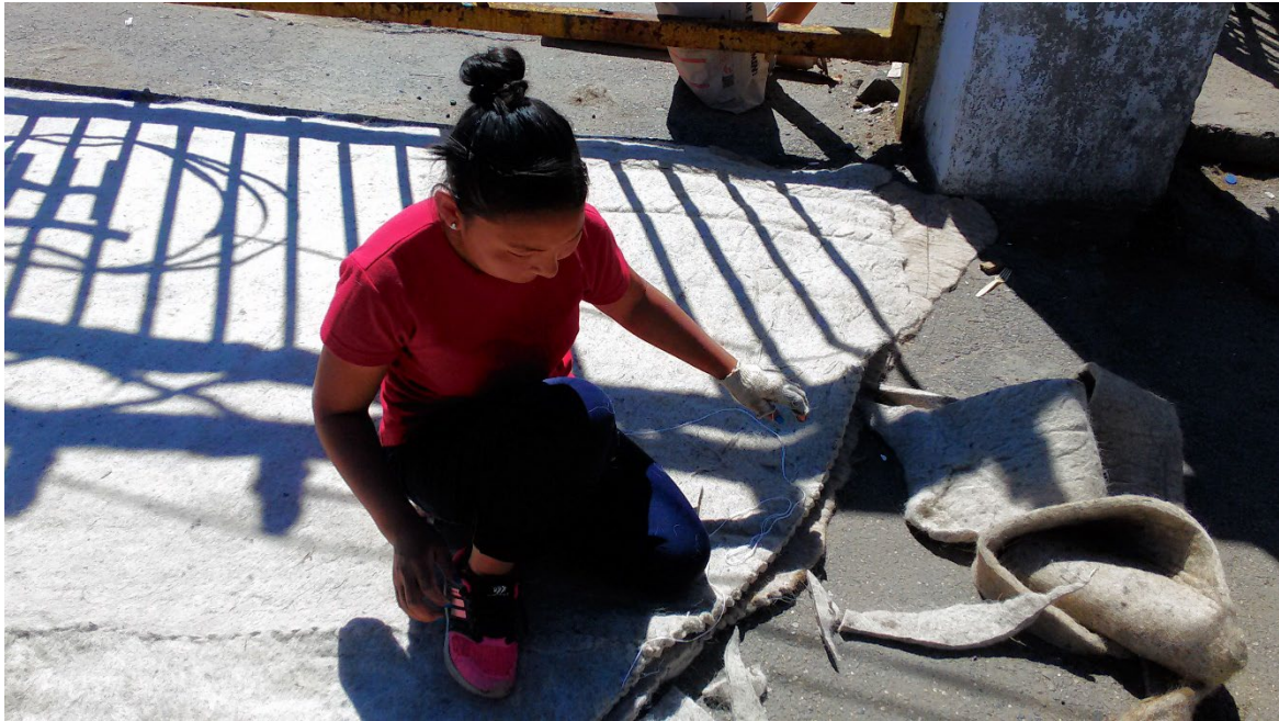
Fig. 2.2 Ger sales at the Narantuul market: (a), (b) images of shops selling gers ; (c) sheets to decorate the interior wall of a ger ; (d) rolled felt sheet; (e) cutting and stitching processes of a felt sheet, which is used as the roof of a ger , in the market
