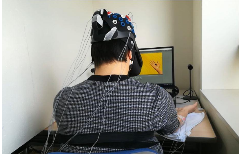
Figure 2.2: Experimental design for motor task performance using the 3D-HMD condition in the VR environment.
