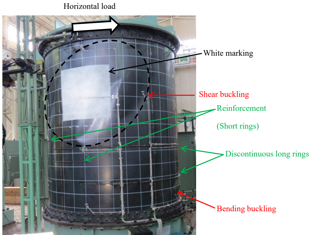
图 3-18 Post-buckling shape of No. (IV) vessel (Horizontal load: 331 kN, displacement: 7 mm, side view)
