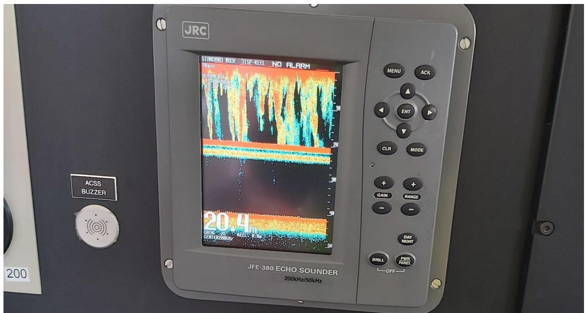
Figure 5-3 Echosounder measurement of water depth from keel
