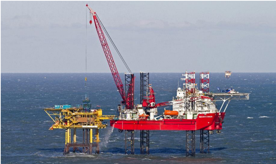
Figure 2-1 Seajacks Kraken Four Leg Jack Up (Courtesy: SEAJACKS)
