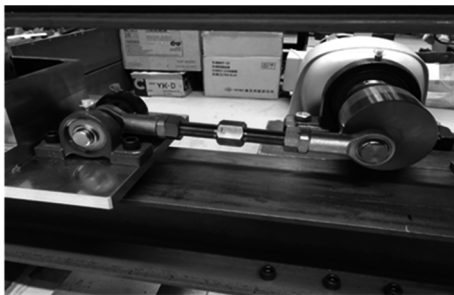
Fig. 2 Overview of the slider-crank mechanism.
