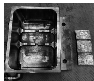
Fig. 6 Overview of the keyway for tank and lower specimen.
