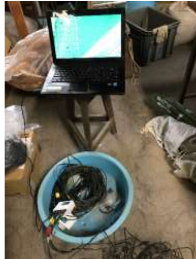
Investigation of moisture sensors and Data-logger's function before application in field measurement
