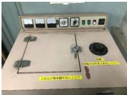
Determination of soil water characteristic curve using Centrifuge Method
