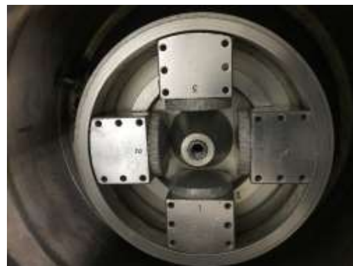
Determination of soil water characteristic curve using Centrifuge Method
