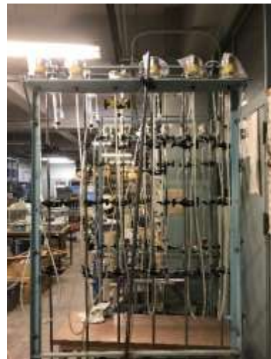
Determination of soil water characteristic curve using hanging column method
