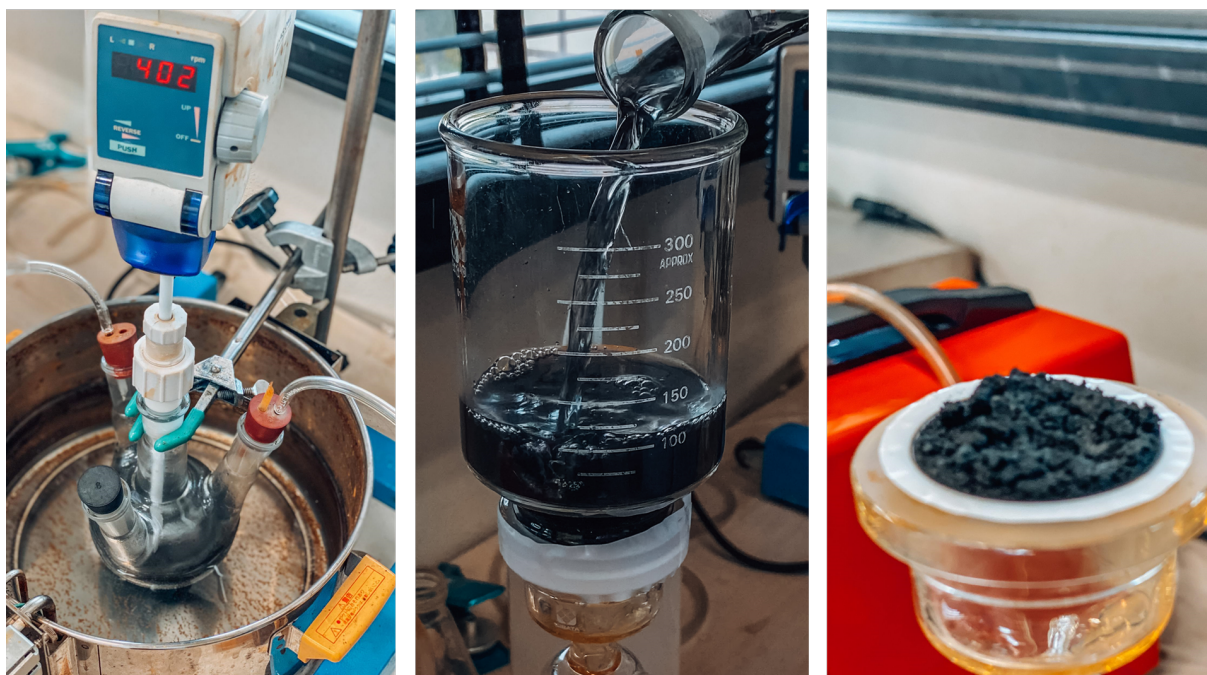
FIGURE 2.9: Synthesis of the Fe 0 -based nanoparticles in the laboratory.
