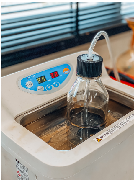
FIGURE 2.10: Ultrasonication (38 kHz, 100 W) and nitrogen gas purging for the preparation of coated iron nanoparticles.
