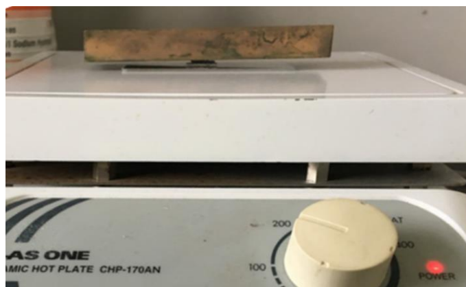
Figure A.2. Experimental setup for transferring MoS 2 onto glass substrate.
