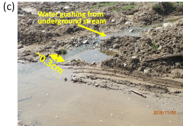
Figure 2.4 Site investigation results from Balaroa: (a) 3D model generated from drone survey. (b) extent of vertical ground displacement and (c) water gushing from underground stream (Survey done on November 3, 2018).
