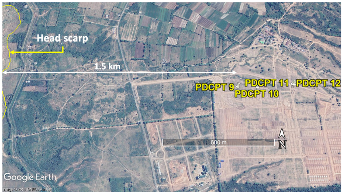
Figure 2.10 Locations of the PDCPTs conducted in the un-failed area, upstream of Jono Oge flowslide site (modified from Google Earth).
