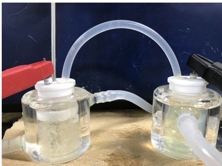
Figure 3-9. Photo of NPs being precipitated (left cell). It is caused by the relative high electrolyte concentration.
