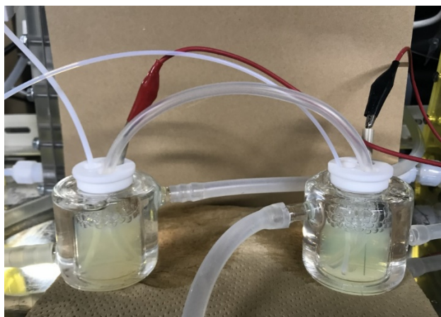
Figure 3-1. Photograph of a bridged thermocell design for open circuit voltage measurement.
