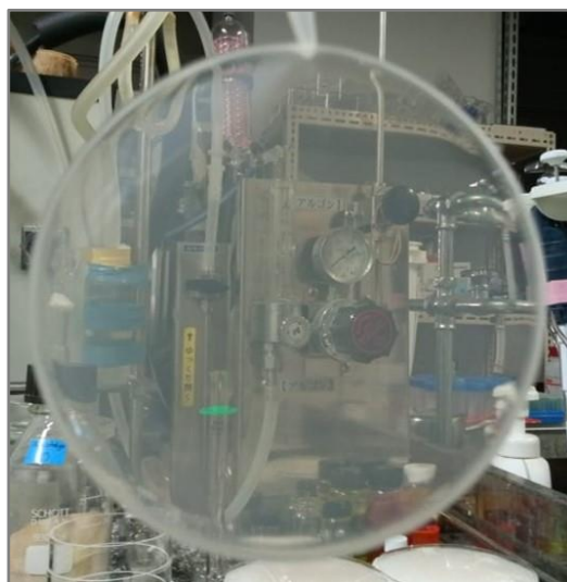
Figure S2.2. PIM with the composition of 50 wt% PVDF-co-HFP, 40 wt% P_{88812}Cl , 10 wt% 2NPOE with total mass of 400 mg.
