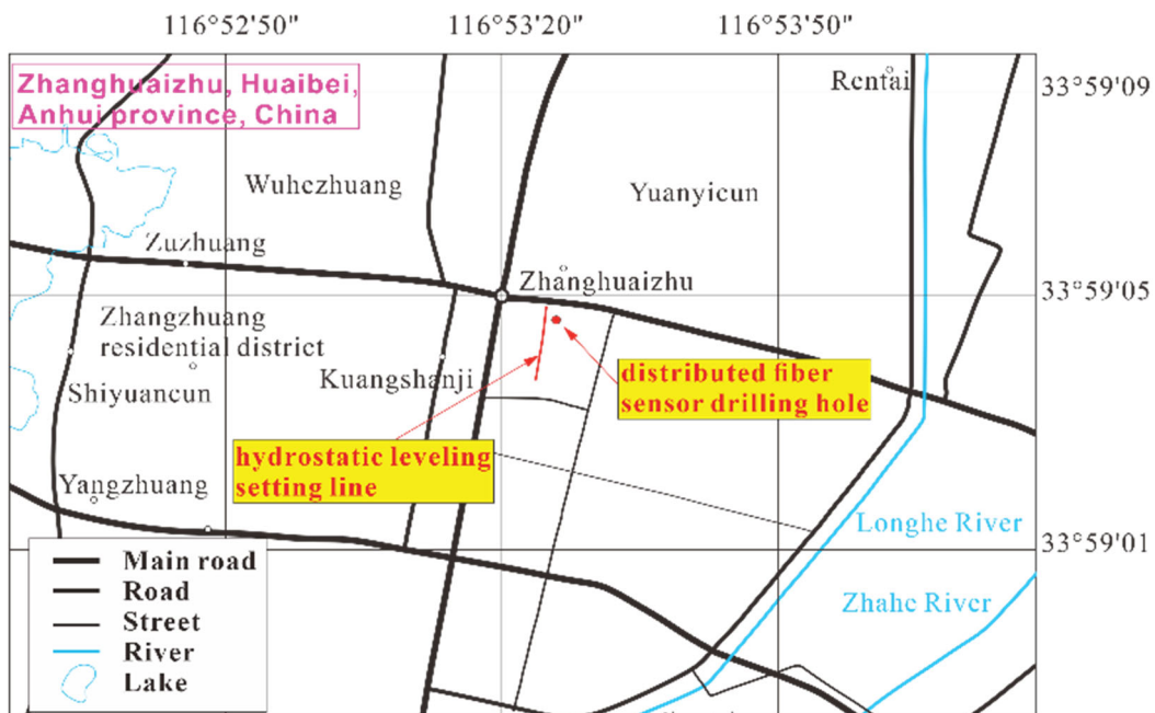
Fig. 3-1 Layout location of hydrostatic levelling line and optical fiber monitoring point
