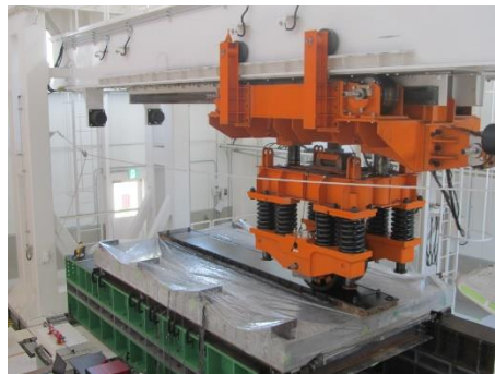
Photo 2. Wheel moving load test machine.
