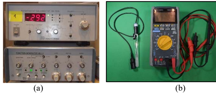
Figure 7. Measuring apparatus used; (a) Galvanostat (b) multi-meter and CSE reference electrode.
