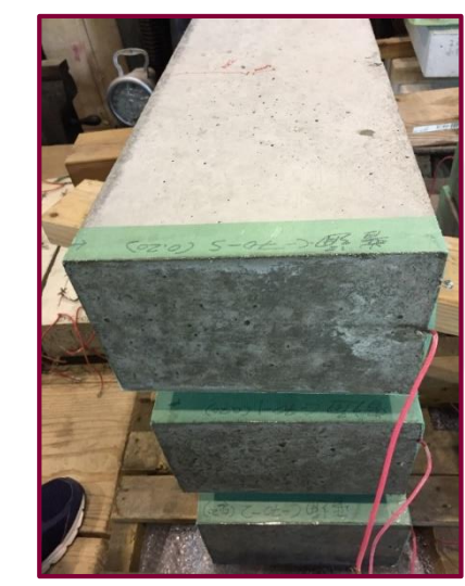
Both ends coated with epoxy
