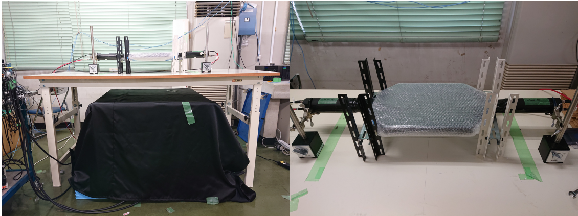
(a) Overview of experimental setup. A cube object covered with black cloth is 2nd gen. muography detector. The Cherenkov detector is placed on a table with height adjustment frame.
