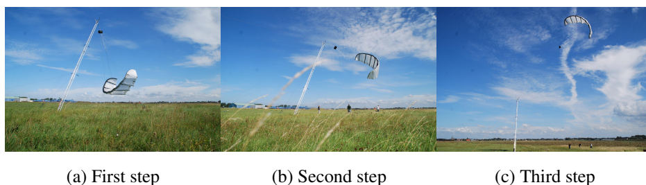
Figure 5.1: Mast launching for soft kites (a) kite is hanged upside down, (b) wind lifts the kite when the mast is going up, and (c) tether is reeled out [13].
