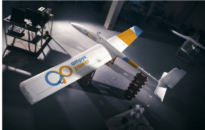
Figure 5.5: A photograph of the AP-2 aircraft developed by Ampyx Power [17].
