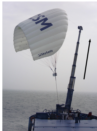
Figure 5.3: Telescopic Mast: Arm extends and lift the kite to a certain altitude [15].
