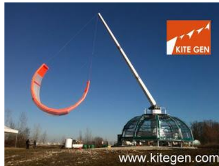
Figure 5.2: Rotational Launch: Kite is connected to a rotating arm, as soon as take-off speed is reached the tether/kite is released [14].
