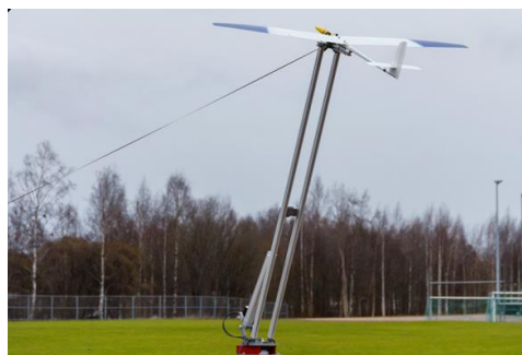
Figure 5.4: Catapult Launch for rigid wing aircrafts, where the system is accelerated using a linear motor [16].
