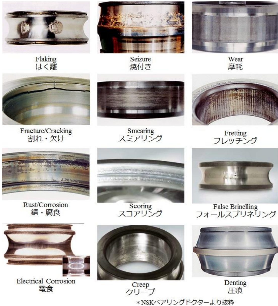
Fig. 1.2 Types of damage in rolling bearing. [3]
