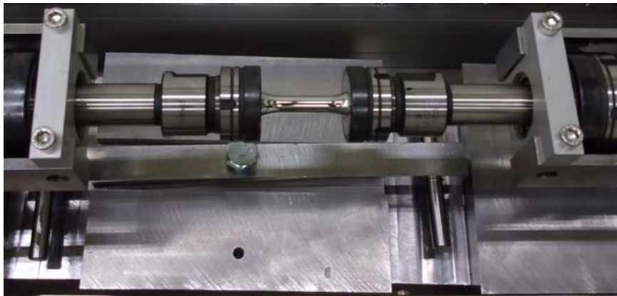
Fig.4-7 Collet chuck for holding specimen.
