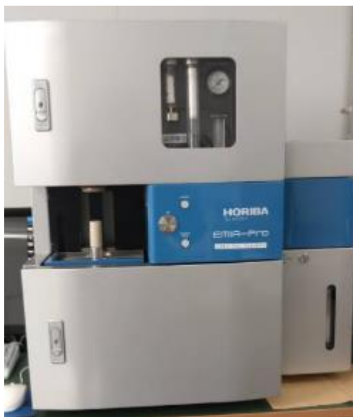
Figure 3.19 Photograph of the machine for the carbon measurement.
