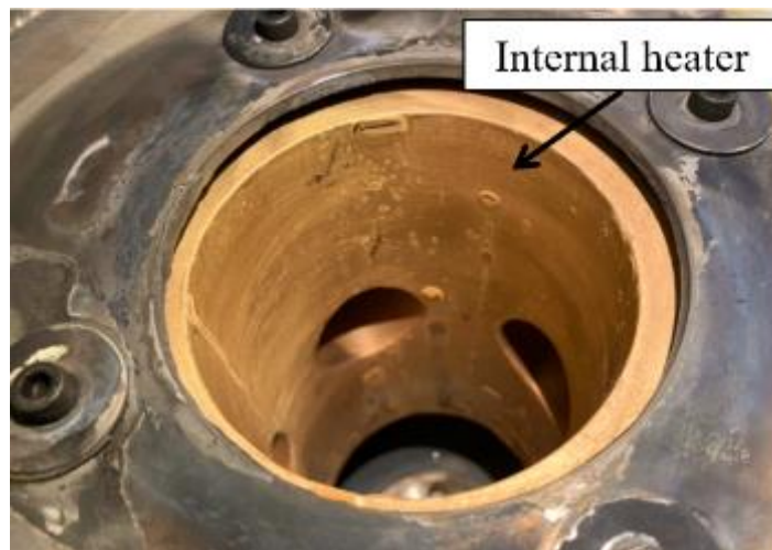
Figure 2.6 Appearance of the brass cast-in heater installed in hydrogen gas chamber after the tensile test in hydrogen at 773 K.
