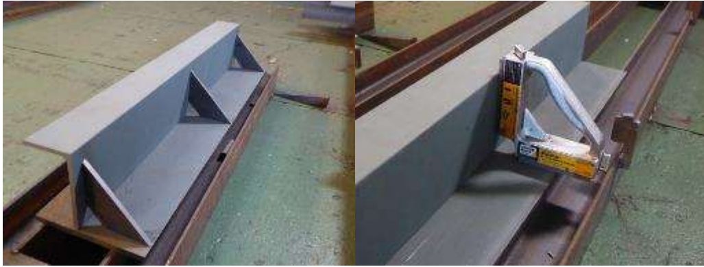
Fig. 3.13 Auxiliary jig using rib piece and magnet clamp
