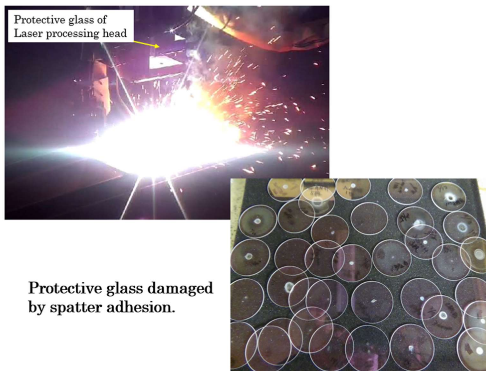
Fig. 3.3 Damage example due to spatter
