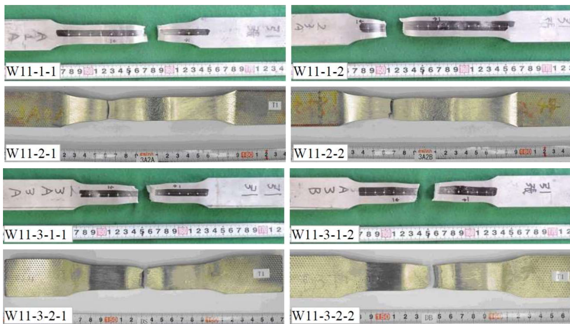
Fig. 3-8 Photograph of specimens made of KSUS329J3L stainless steel after tensile tests.
