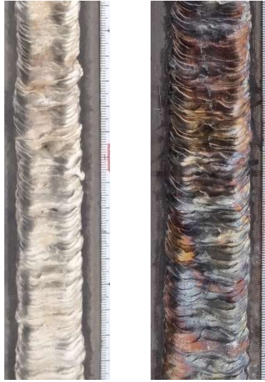
Fig. 2-4 Examples of scale beads for butt weld joints produced by vertical upward welding
