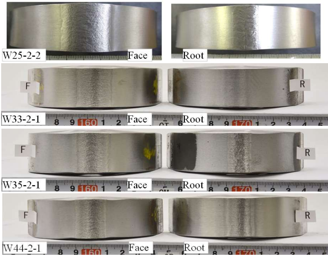
Fig. 4-6 Photograph of specimens made of various combinations of base metal after bending tests.
