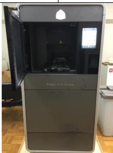
Figure3.1.1 ProJet3500 HD Professional 3D Printers
